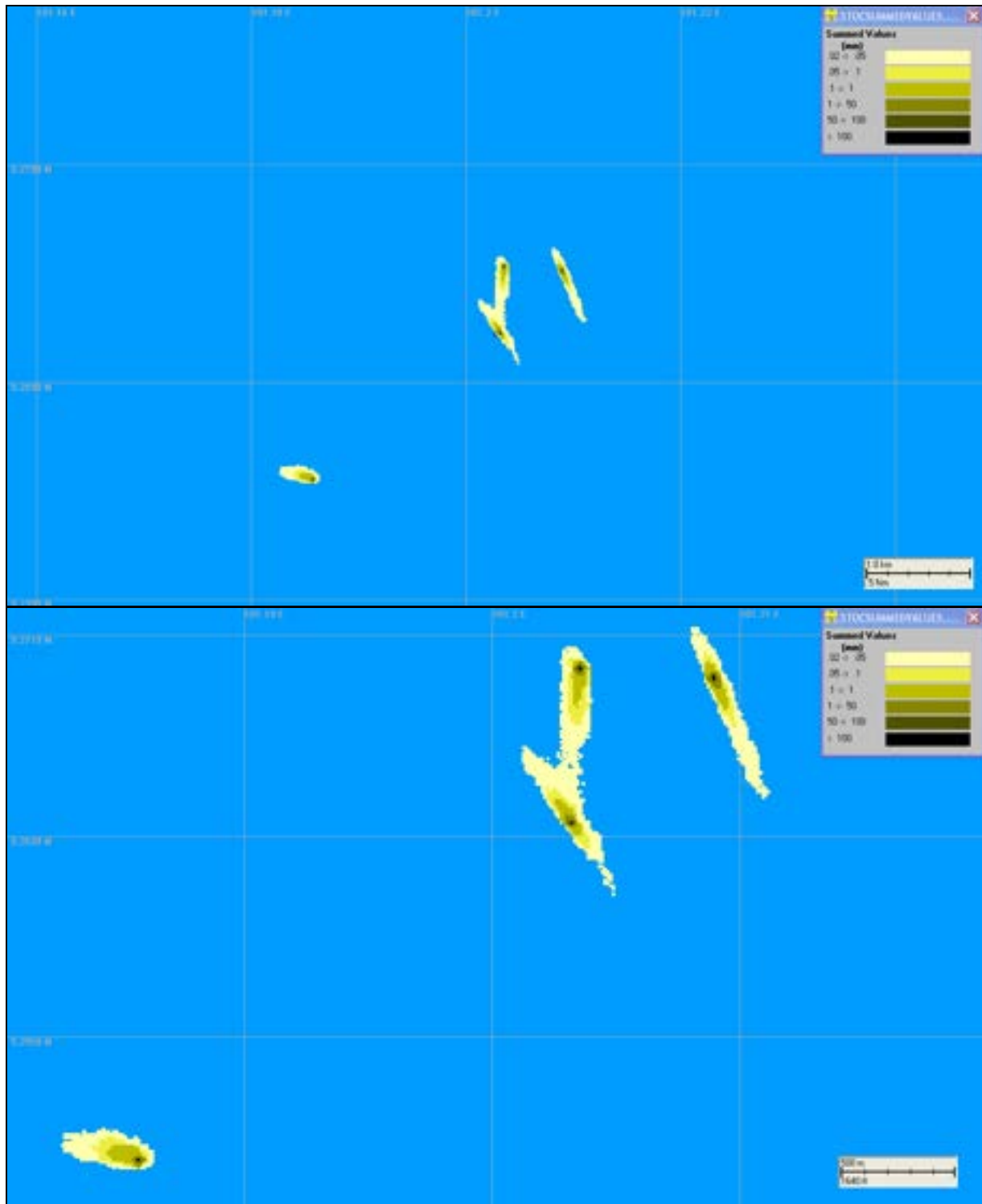
Figure 14: Sample figure showing large scale view (top) and zoomed-in view (bottom) of the predicted bottom and seabed coverage of cuttings released near the seabed for all four wells during January current conditions.
